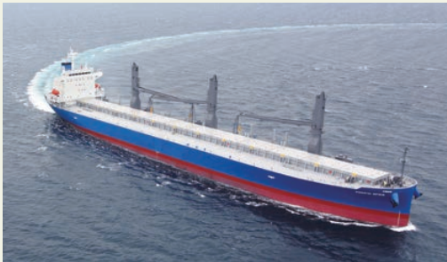
“Pacific Spike” for transporting long rails allows a reduction in welding operations of rails locally, contributing to the reduction of time and costs.
