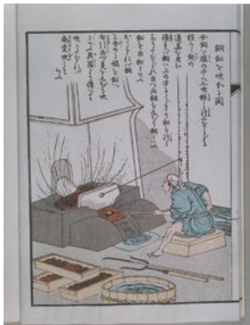
Sumitomo's original copper refining method
