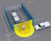
Mobile hydrogen station equipped with a simple dispenser
