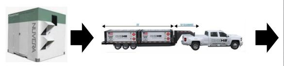
Hydrogen production using a compact gas reformer
