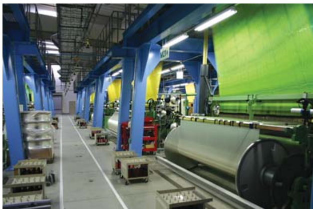
High-speed Jacquard loom at Sumisho Airbag Systems' state-of-the-art side-curtain air bag factory in Nagasaki. The factory began shipping in January 2006, and has an annual production capacity of 1.2 million bags. We are enhancing production capacity with the aim of reaching full production at around 4 million bags per year.
