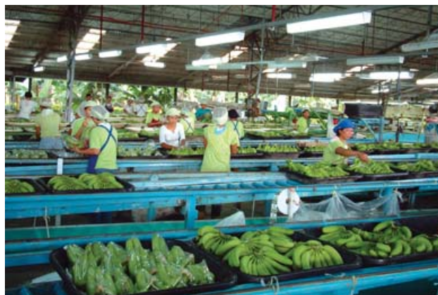
Sumifru's fruit packing facility at Davao in the Philippines. Bananas are being inspected for quality in line with strict Japanese standards, divided into bunches suitably sized for retail sale, and packed for shipment. We have an established delivery system for high quality products, including chilled shipping.
