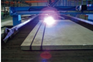
Laser cutting line for stainless steel plates at KCCMTI. In China, demand for stainless steel used in construction and infrastructure development and for machinery manufacturing is increasing. We are working to develop and cultivate new demand by taking full advantage of KCCMTI as a steel processing and sales base.
