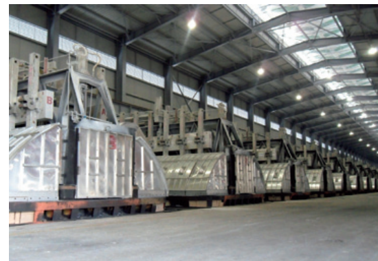
▶ Electric furnaces for smelting aluminum ingots at Press Metal Berhad in Malaysia
