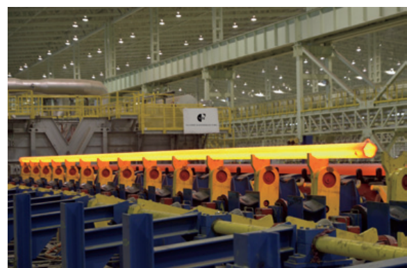
▲ Small-diameter seamless steel pipe manufactured at Vallourec Star, LP in the U.S.
