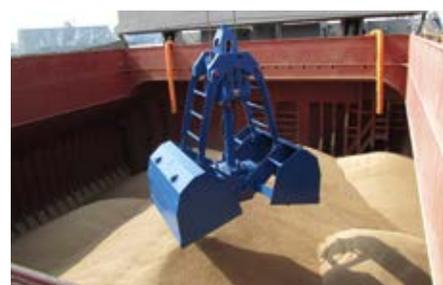
Unloading of wood pellets, a biomass fuel
