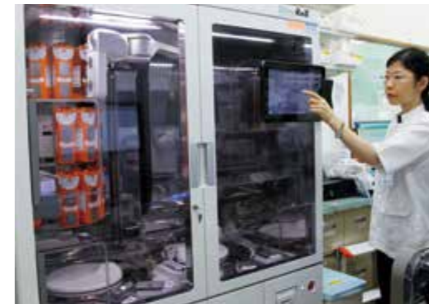
Fully automated dispensing equipment
