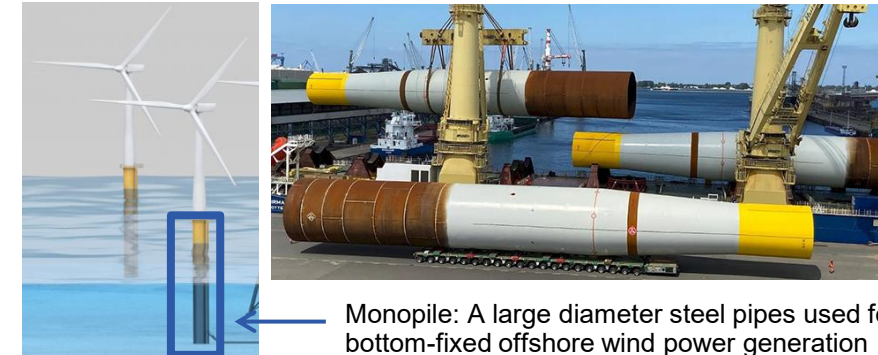
Monopiles being loaded at EEW quayside in Rostock, Germany
