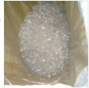
Flaked PET bottles processed with an RVM
