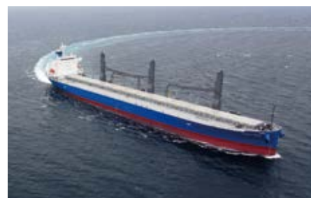
Specialized vessel for transporting long rails
