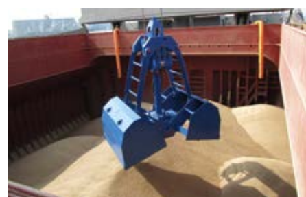
Unloading of wood pellets, a biomass fuel
