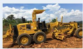
Training of local operators of supplied machines The vehicle in the photo is a motor grader used for ground leveling
